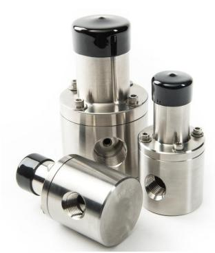
**Griffco BPMP-Series** diaphragm back pressure valves are designed to enhance the performance of chemical feed systems by applying a continuous back pressure to the chemical feed pump, while also acting as an anti-syphon valve. Robust construction ensures reliability in the rigorous service of municipal and industrial applications. Wetted materials include: **316 SS, A20, Hast. C**, and **Titanium.** Available sizes: '4" – 1".
