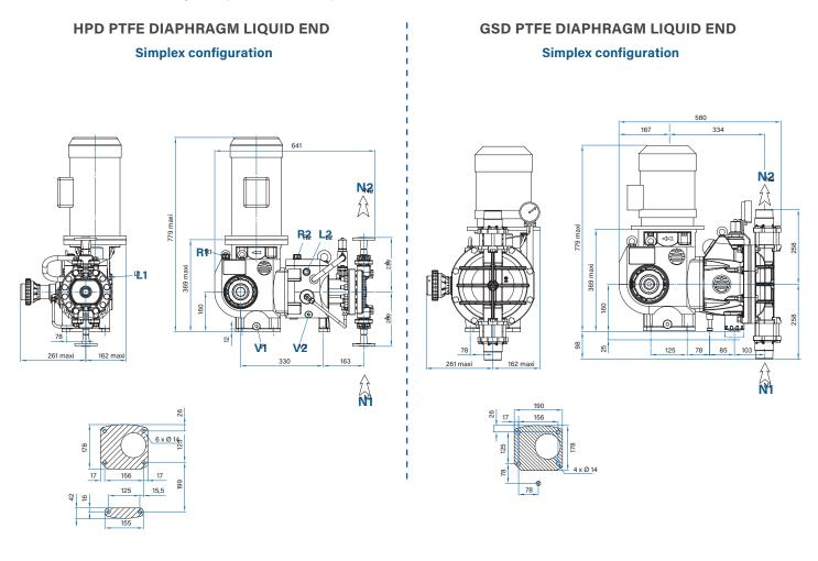
N1 Suction - N2 Discharge - V2 Drain hydraulic oil - L2 Hydraulic oil level - R2 Hydraulic oil filling - V1 Drain mechanic oil - R1 Mechanic oil filling - L1 Mechanic oil level oil level
